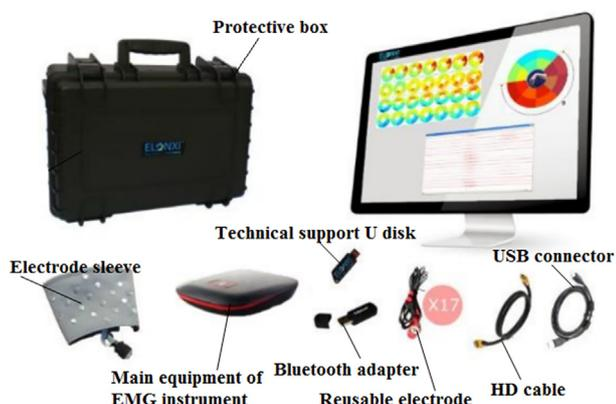
Fig. 2 Experimental equipment.
